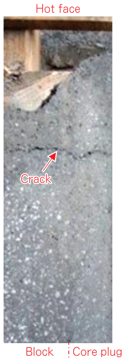
Fig. 5 Cut section of used MHP.
