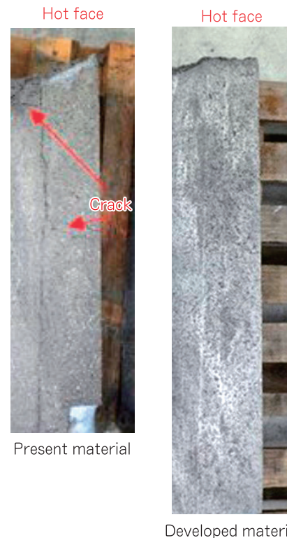
Fig. 17 Cut section of present material MHP and developed material MHP after use.
