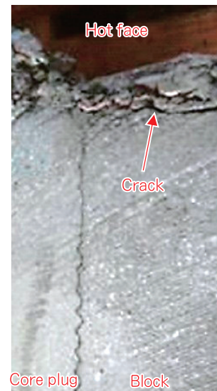
Fig. 3 Cut section of used large mono-block MHP.
